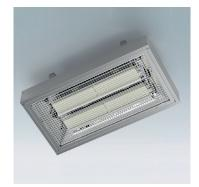
4 Ceramicx FTE Ceramic Elements Grill Protected Element Colour White Stainless Steel Body Aluminised steel reflectors Panel size 750 x 400 x 110mm -11kg Heating Up Time < 5 Minutes Useful Wavelength Range 2-10 μm IP Rating: IP20
