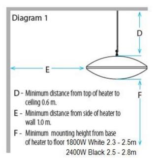
The Herschel PULSAR must be located in a position to allow proper and efficient use but one that ensures hot parts are not touched accidentally. The recommended installation height of the White 1800W Pulsar is 2.3m-2.5m~(90"-110") from the floor.
